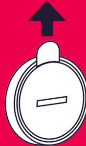
Remove the plastic tab to put the Remote Control in pairing mode. The LED on the front will start blinking once per second.\*
