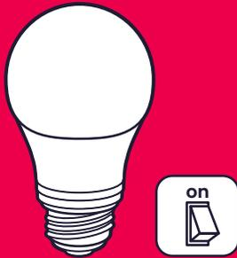
Turn the light off for at least 5 seconds using the wall switch and turn it on again. The light is in pairing mode for 1 minute from now.
